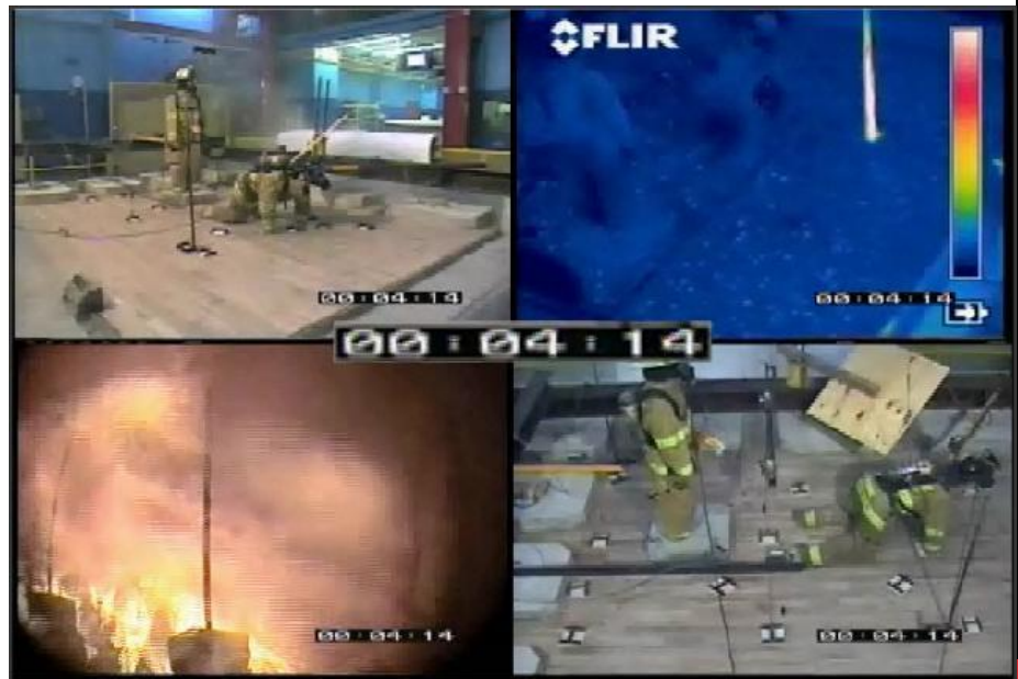
FIGURE 4: UPPER RIGHT THERMAL VIEW – COLD FLOOR LOWER LEFT HEAVILY INVOLVED BASEMENT FIRE BELOW THE FLOOR
